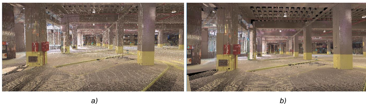
Figure 10 – Point cloud before (a) and after (b) the different surface tonalities are eliminated
