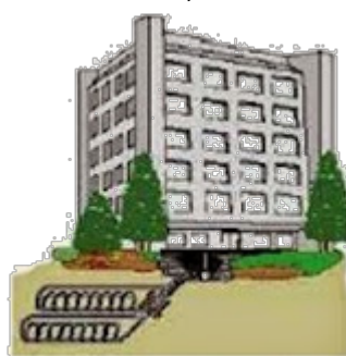
Graphic 11: Horizontal closed loop.
