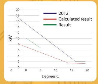
The blue line is a power signature developed from 2012 data, the red line is a theoretical power signature for the building's heat after the actions was performed and the middle green line is the actual outcome of the energy use.
